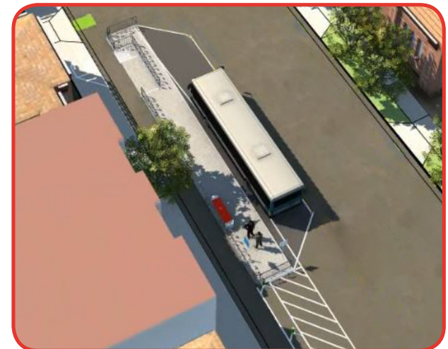
Bus Stop Island, Street Resurfacing
